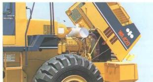
**Tilt-back engine hood:** With generous footholds and access the mechanic can easily make engine checks, replace parts and perform orther required maintenance.
