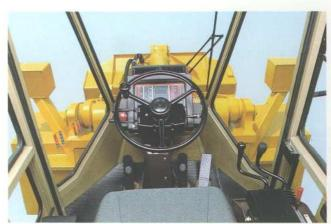
Operator's cab: Designed and laid out for maximum comfort and efficiency, the cab offers a wide field of vision, plenty of work space and ergonomically arranged instruments, levers and pedals. Vibration and noise are also kept to a minimum. The adjustable steering wheel tilts within a 100 mm (4") range for operating convenience. The suspension seat is fully adjustable for maximum operator comfort.
